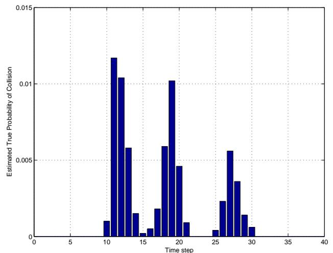
Fig. 7. Estimated true probability of collision for each time step in a typical plan where  $\Delta = 0.1$ . The highest probability of collision is still significantly lower than  $\Delta$ , indicating significant conservatism in the plan.
