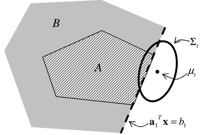
Fig. 2. Predicted distribution of  $X_t$ , shown as mean  $\mu_t$  and covariance ellipse  $\Sigma_t$ , in relation to obstacle. The probability of satisfying the constraint  $\mathbf{a}_i^T X_t < b_i$  is the integral of this distribution over the region  $A \cup B$ , which is greater than or equal to the integral over the region  $A$ , the probability of collision.
