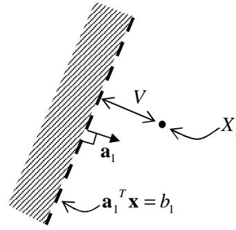
Fig. 4. Linear constraint and vehicle position  $X_t$ .  $V$  is the distance between the constraint and the vehicle, defined as positive for values of  $X_t$  for which the constraint is satisfied, and negative for value of  $X_t$  for which the constraint is violated. The vector  $\mathbf{a}$  is the unit normal in the direction of positive  $V$ .
