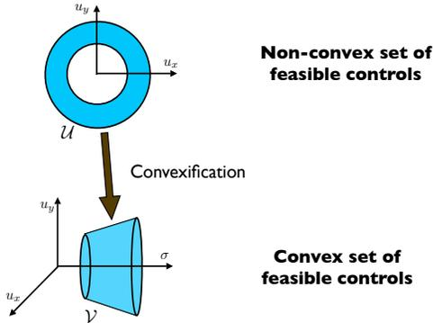
Fig. 2. Convexification of the Control Magnitude Constraint for Soft Landing. The annulus represents the actual non-convex control constraints in  $(u_x, u_y)$  space, which is lifted to a convex cone in  $(u_x, u_y, \sigma)$  space for the RCP (5).
