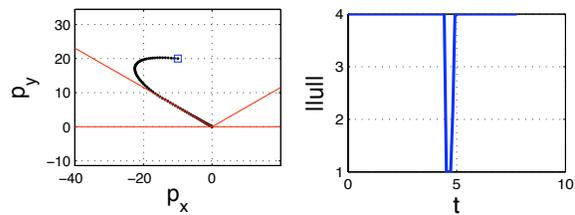
Fig. 5. *Minimum fuel trajectory on the boundary:  $u(t) \in \mathcal{U}$  for all  $t \in [t_0, t_f]$ . Lossless convexification via Theorem 3.*
